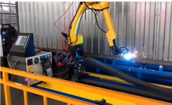
Automatic welding robot
